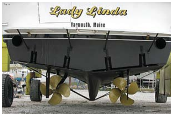
HOT WHEELS. ZF's high-tech Faster Propellers' progressive pitch and airfoil shape squeeze another 5 percent or more from each drop of fuel.
