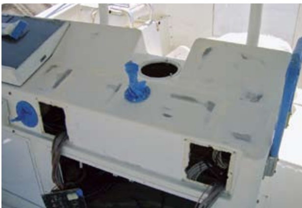
EXTREME MAKEOVER. Lady Linda's dated helm (top left) is filled and painted and then fitted with new Cummins MerCruiser Diesel SmartCraft electronic gauges and Digital Throttle and Shift controls. This 1981 Hatteras 50 was repowered with Cummins QSM-11 diesels.
