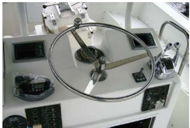
EXTREME MAKEOVER. Lady Linda's dated helm (top left) is filled and painted and then fitted with new Cummins MerCruiser Diesel SmartCraft electronic gauges and Digital Throttle and Shift controls. This 1981 Hatteras 50 was repowered with Cummins QSM-11 diesels.
