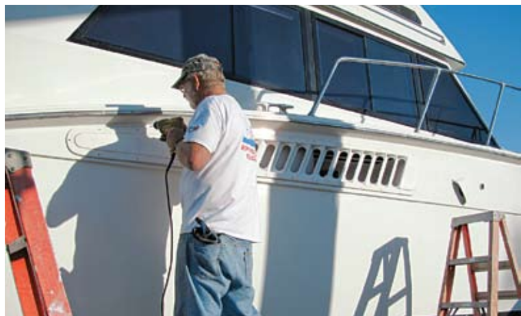
AIR IT OUT. Large hull-side vents into Lady Linda ’s engine room provide air for the new engines’ increased horsepower but keep seawater out.
